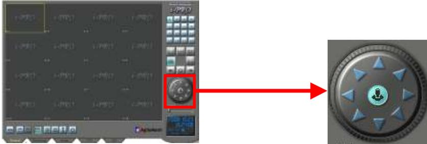
Pan and Tilt functions are available for Pan/Tilt control capable cameras connected to the Camera 1 or Camera 2 input on AgileMesh AV7510 or AV7520 tactical nodes. The AgileMesh nodes use RS-485 differential pair for PTZ control. The default protocol setup is Pelco-D, 2400 baud, 8 data bits, no parity and 1 stop bit. A green “P” will appear in the upper right corner of a viewing window if the node has been setup for PTZ controls.
