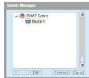
Additional cameras can be added by a single-click to “SWAT Cams” (this will highlight it). Next right click the highlighted “SWAT Cams” and select “New Site” which will bring up the “Server Add” configuration box. Refer to **Appendix 1** for the camera IP addresses and video port numbers. Click “OK” to add the second camera.
