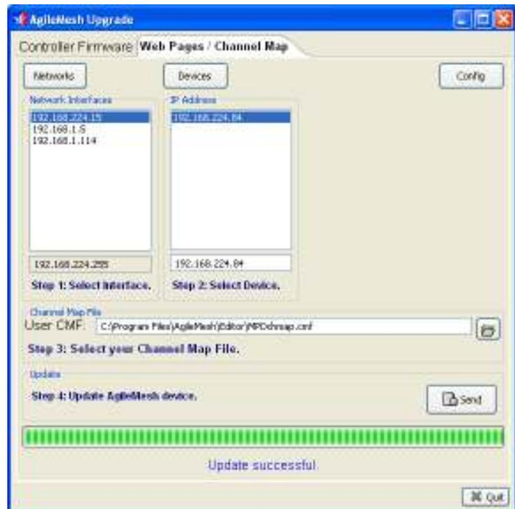
Restart the target node by turning power off and back on. When the Channel and Neighbors indicators stop flashing (after about a minute and a half), turn the channel knob to the desired channel. **Note: you must change the channel for the new settings to be used. If the channel displayed is the one you want to use, turn the channel knob to the next channel and then back immediately.**
