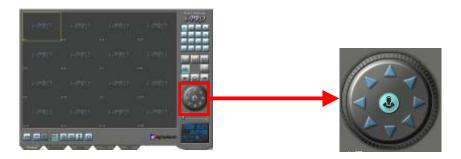
Pan and Tilt functions are available for Pan/Tilt control capable cameras connected to the Camera 1 or Camera 2 input on AgileMesh AV7510 or AV7520 tactical nodes. The AgileMesh nodes use RS-485 differential pair for PTZ control. The default protocol setup is Pelco-D, 2400 baud, 8 data bits, no parity and 1 stop bit. A green "P" will appear in the upper right corner of a viewing window if the node has been setup for PTZ controls.
