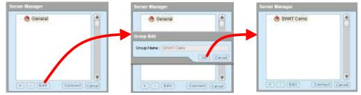
"SWAT Cams". Single- click "SWAT Cams" to highlight it. Next right click the highlighted "SWAT Cams" and select "New Site" which will bring up the "Server Add" configuration box. Select a name for the camera to enter for "Server Name". Camera IP addresses are set by the Node knob
