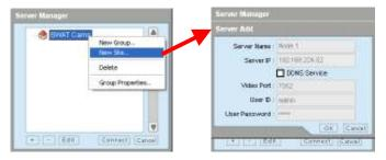
on the front panel of the AgileMesh equipment. In this example, the "Server Name" will be "Node 1". The IP address for a camera connected to Node 1 is 192.168.224.52 and is entered in "Server IP". "DDNS Service" is
