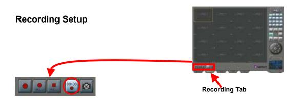
Click "Schedule Recording" Button in the Recording Tab to set up the automatic schedule recording function of each channel with assigned date & time.
